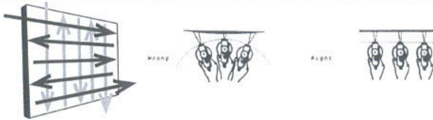
Figure 3. Proper spray application of L-B-C Lead Barrier Compound
