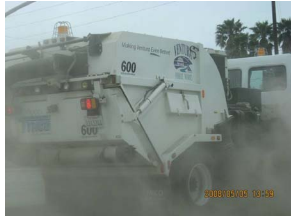
Figure 6. Example of street sweeper in violation of proposed operational standard.
