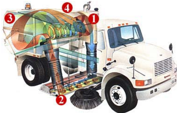
Figure 5: PM-10 certified street sweeper with enclosed air recirculation and cyclone particulate trap.
